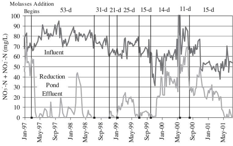
**Figure 1** Nitrate+nitrite concentrations in the Mode 2 Reduction Pond. Hydraulic residence times in days are shown
