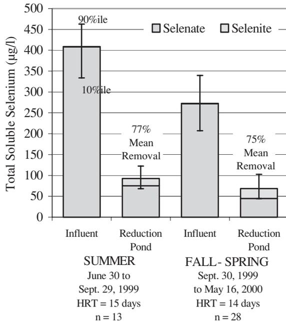
**Figure 2** Mean soluble selenium reduction by Mode 2 RP
